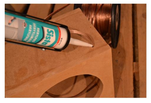
**Fig 8.** Speaker cable mounted and closed with sealant so that the structure is fully sealed.
