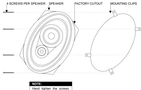
in a crisscross pattern to avoid bending the speaker basket or stripping screws.
