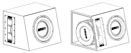
Two 10-inch subwoofers + one PUMP-12 Two 12-inch subwoofers + one PUMP-12
