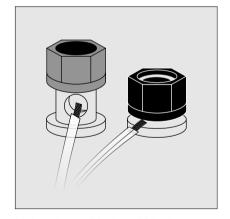
Using the gold-plated binding posts: you can easily connect banana-plugs, spade-plugs and bare wire. Insert the wire into the hole tighten securely (do not let bare wire hang out side of hole).
