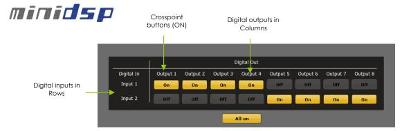
Note how labels of input channels and output channels followed on the Matrix mixer to simplify your routing. Let's illustrate the concept of configuration of this block using a 3way configuration + 2 subs where both Left & Right signals are being mixed (combined).
