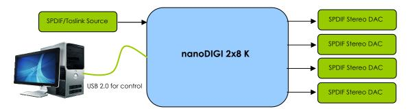
Being an all digital platform, the nanoDIGI only interfaces to SPDIF/Toslink digital audio interface.
