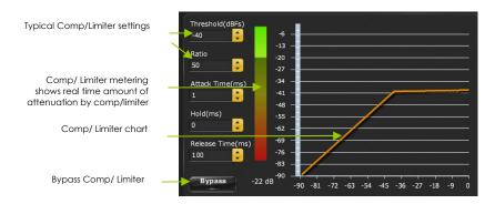
A compressor/Limiter allows dynamic range compression of the signal to prevent damage of your speakers. Extensive information is <u>available online</u> on the use of compressor/limiter. Please take the time to familiarize yourself with such processing block before using it.
