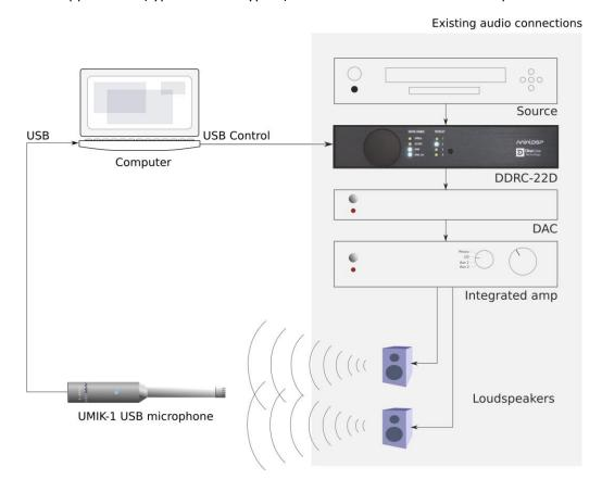
Place the UMIK-1 microphone into the microphone stand and point it between the speakers. Position the computer and cabling so that there is enough freedom of movement to move the microphone into the needed locations.
