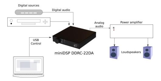
Computer connectivity is used to perform acoustic measurements and generate digital room correction filters. Up to four sets of correction filters can be stored on the *Dirac Series* processor and recalled from the front panel or via an infrared remote. Once the processor is fully configured, the computer is no longer needed.
