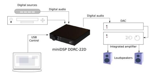
The DDRC-22DA (digital input/ analog output) is typically inserted between digital sources and a power amplifier, as illustrated below.
