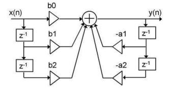
A single biquad like this can perform a great many functions, including all of the functions of a single parametric EQ filter, one 6 or 12 dB/octave high pass or low pass filter, and more. Biquads are combined in series (cascaded) to create more complex filters. The function that each biquad performs is determined by just five numbers: *a1*, *a2*, *a0*, *b1*, and *b2*. These numbers are called the *coefficients*.
