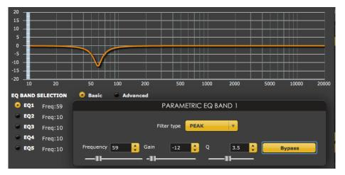
Dips in the frequency response can be treated with a corresponding peak filter, but care should be taken not to use too much boost or to use high-Q filters. Too much boost can cause signal clipping, and narrow dips are typically caused by acoustic cancellations in the room and cannot be removed with EQ.
