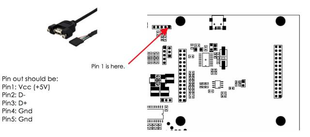
This header will interface to common off-the-shelf cable assemblies (typically used in computer hardware). Although this is a standard connector, you should nonetheless confirm the pin-out with the manufacturer, or you could easily cause damage to your computer or 8x8 Kit. In most cases, pins 4 and 5 can be identified by a black wire, but once again, DO check the manufacturer's spec of the connector to prevent any short-circuits.
