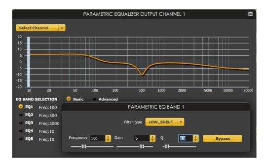
There are six parametric EQ filters on each input and output channel. The window displays a frequency response graph showing the combined response of all enabled parametric filters on that channel. For example, the screenshot above shows a response curve created with a low-shelf boost filter at 100 Hz, a dip at 500 Hz, and a high-shelf cut filter at 5000 Hz.
