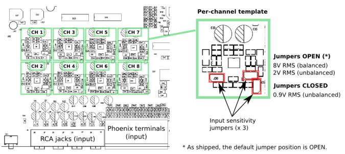
Do not make a balanced connection to the input of any channel with jumpers in the CLOSED position.
