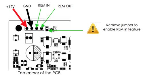
This Phoenix connector also has terminals for remote enable/disable. Remove the jumper as shown above to enable this feature.
