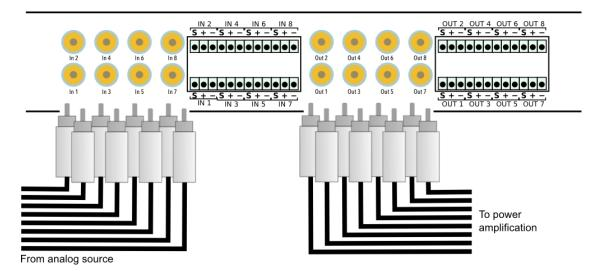
Balanced connections are made by connecting bare wire ends to the push-in Phoenix terminal blocks. For advice on using these, see <u>Balanced wiring tips</u> on page 46.
