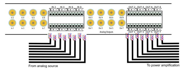
If using a mix of balanced and unbalanced connections, be aware that you cannot connect an input both ways. That is, for any given input channel, connect either to the RCA jack, or to the terminal block, but not both.
